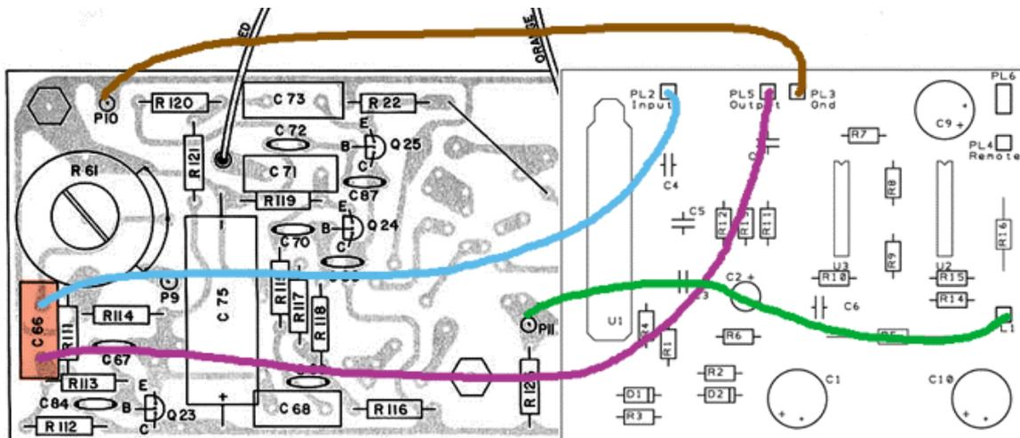
Wiring is very easy (only four wires), but some soldering necessary. C66 (marked red) has to be removed before inserting and soldering of input/output wires into circuit board holes. Be careful not to short-circuit the MIG-L power plane with the screw/bolt.
