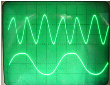
The MIG-L resembles the sound of an overdriven Leslie 122 amp perfectly. It produces a smooth clipping (lower curve) which is a little more rounded than the 122 amp's cut to emulate somewhat "used" tubes. As you can see, even the distortion product (upper curve) comes very close to the original. You can even modify the MIG-L to get a "new tubes" sound with a clipping exactly as pictured above, if you prefer.
