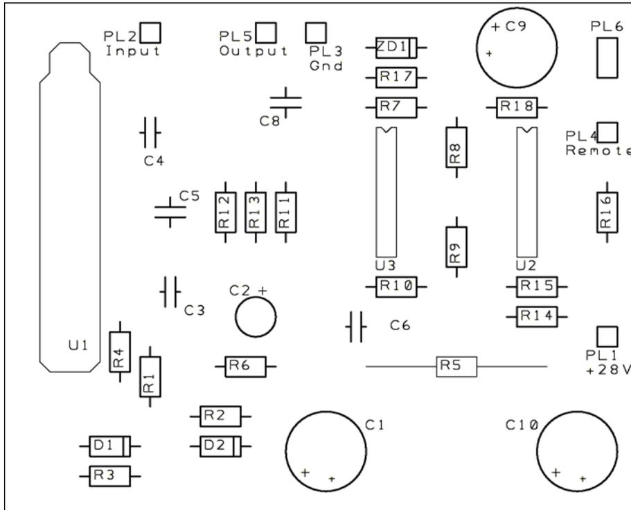
**Board layout of MIG-L printed circuit board**
