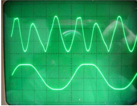
An overdriven Leslie 122 amp (this one equipped with new Electro-Harmonix 6550) produces a smooth round clipping above the amp's power margins (lower curve). The upper curve (done by a distortion analyzer) shows the distortion product. As you can see, most of the "overdrive condition" distortion is "k3" (three times the frequency of the 1 kHz test signal).
