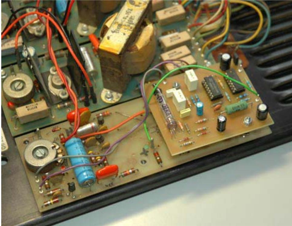
This is a MIG-LR affixed to a Leslie 760 amplifier panel. To the left you can see the Gain and Volume potentiometers. I have drilled them and glued a long M4 screw as an axle into the hole for easier access. The MIG-L board measures 80 x 65 mm; screw holes fit well above the crossover board so it can be mounted on top with two 6-32 UNC 1" screws and two 15 mm plastic spacers. Be careful not to short-circuit the MIG-L power plane with the screw/bolt.
