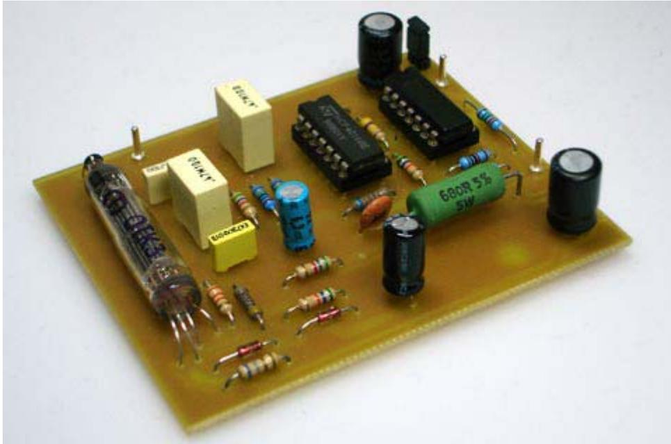
**The MIG-L Leslie Tube Overdrive works with a real miniature tube. The MIG-LR even has a remote control input for switching between tube limiter and bypass mode.**
